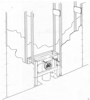
Pan only with cistern mounted within wall linings.
